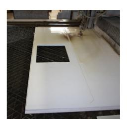
Do the entry hole outside respect the slab. In alternative make the hole a few centimeters from cutting perimeter and in any case, never less then 5mm. For inner holes, do always the input and output hole internally respect the part that you want to cut. Follow the below diagram (a low pressure for entry hole)
